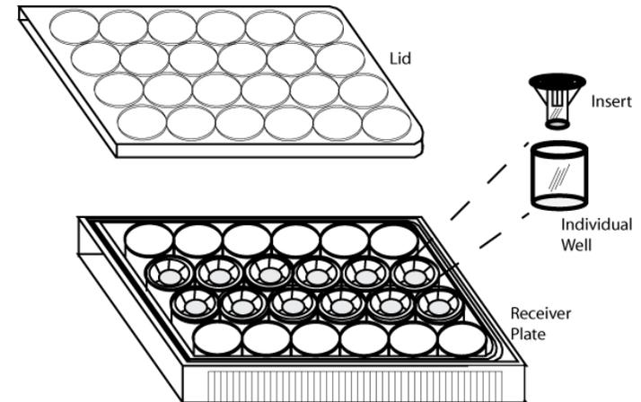
Figure 3. Diagram of 24-Well Cell Invasion Chamber.
